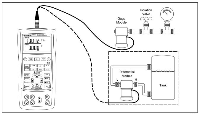
Figure 13. Connections for Measuring Pressure
