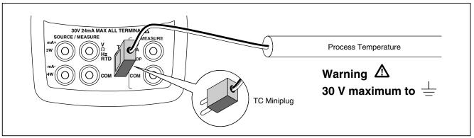
Figure 10. Measuring Temperature with a Thermocouple
