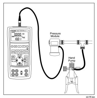
Figure 18. Connections for Sourcing Pressure
