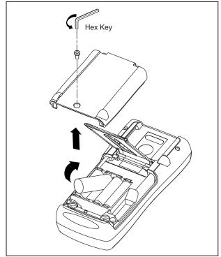
Figure 23. Replacing the Batteries
