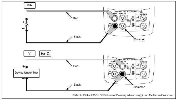
**Figure 15. Electrical Sourcing Connections**
