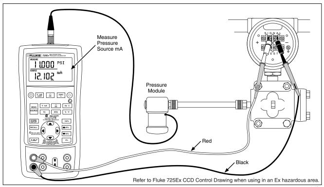
Figure 21. Calibrating a Current-to-Pressure (I/P) Transmitter
