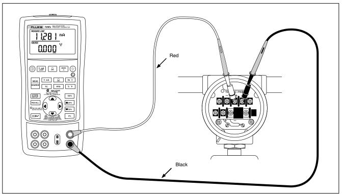
Figure 8. Connections for Supplying Loop Power
