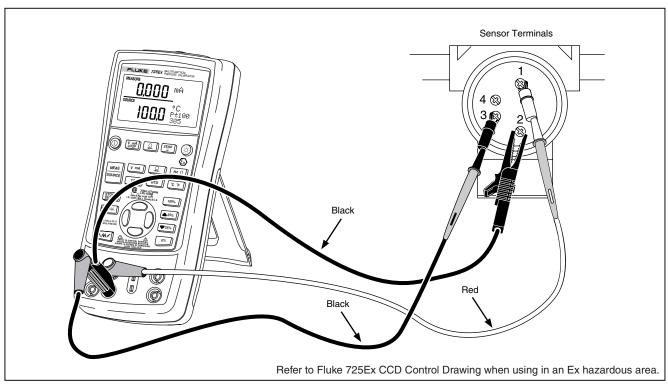
Figure 17. Connections for Simulating 3-Wire RTD
