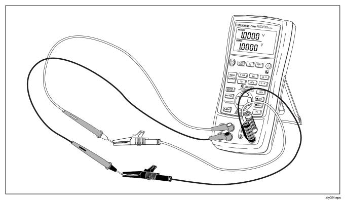
Figure 5. Voltage-to-Voltage Test
