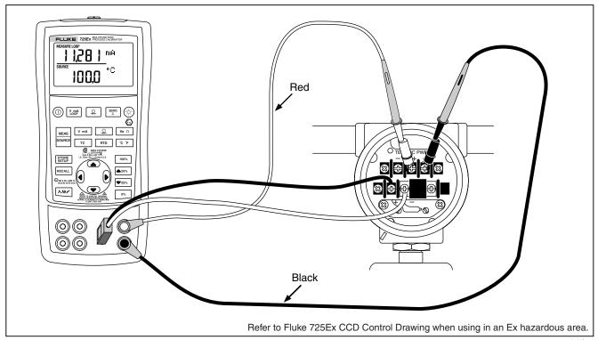
Figure 19. Calibrating a Thermocouple Transmitter
