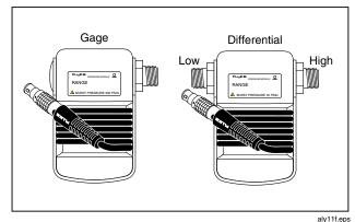
Figure 12. Gage and Differential Pressure Modules
