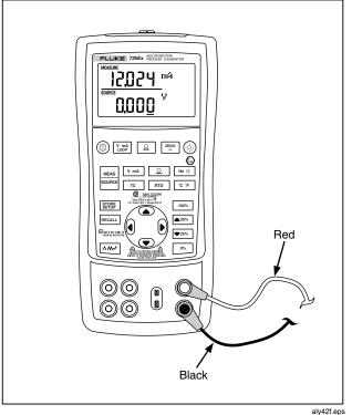
Figure 7. Measuring Voltage and Current Output
