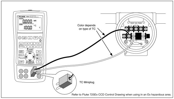
Figure 16. Connections for Simulating a Thermocouple
