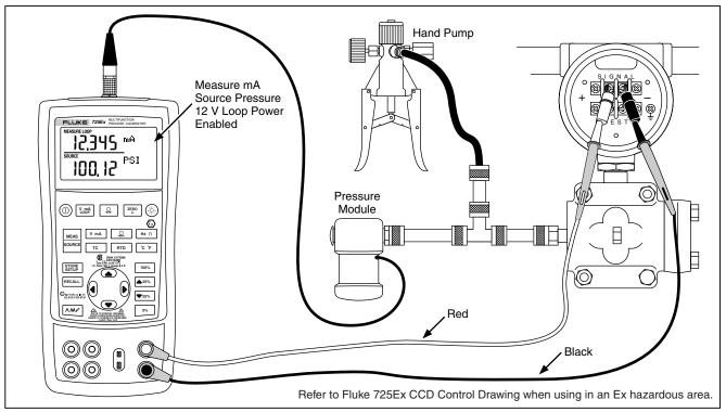
Figure 20. Calibrating a Pressure-to-Current (P/I) Transmitter
